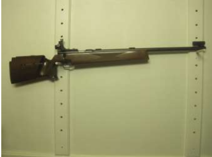
67. Anschutz Target Rifle mod. Match 54 22 LR cal bolt action rifle w/target sight & double set trigger ser # 78163
