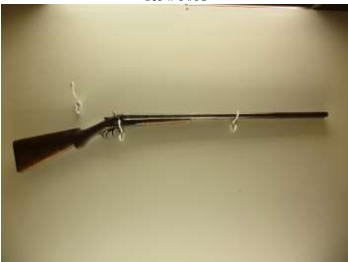
40. St. Louis Arms Co mod. SXS 12 ga double bbl shotgun Belgium Laminated Steel hammered ser # 190891
